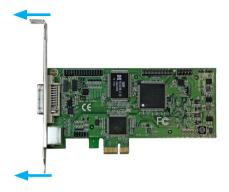
d) Line up your desired bracket so that the DVI input-port, and the A/V breakout cable input-port align with the port holes. Also ensure the screw hole is aligned with the underside of the PEXHDCAP60L.
